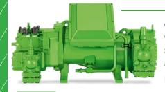
All ElectraTherm ORC systems are powered by BITZER's semi hermetic, twin screw expander. This allows ElectraTherm's ORC process to utilize much more variable heat sources than leading turbine technologies thanks to greater transient operation that allows for "wet" dual-phase flow and greater turndown ratios allowing for continuous power generation when dealing with inconsistent thermal input.
